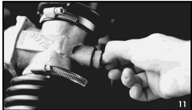
mixer improved thanks to the gas pipe motorization through a stepping engine adapted on the basis of the BLOS. The signals sent out by the Lambda oxygen sensor are analysed by the Ecogas Junior or Ecogas ECU which, through the stepping engine, controls the gas pipe rise or descent, then the mixture leaning out or enrichment. The carburation has permanently and automatically an optimum mixture.
